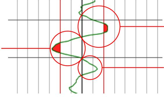
When the graph is below the centreline, the deviation is below the mean line.
