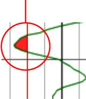
Where the graph is coloured red, the limits of the specification have been exceeded. The whole run fails to comply with the specification if any part of the graph is coloured red.
