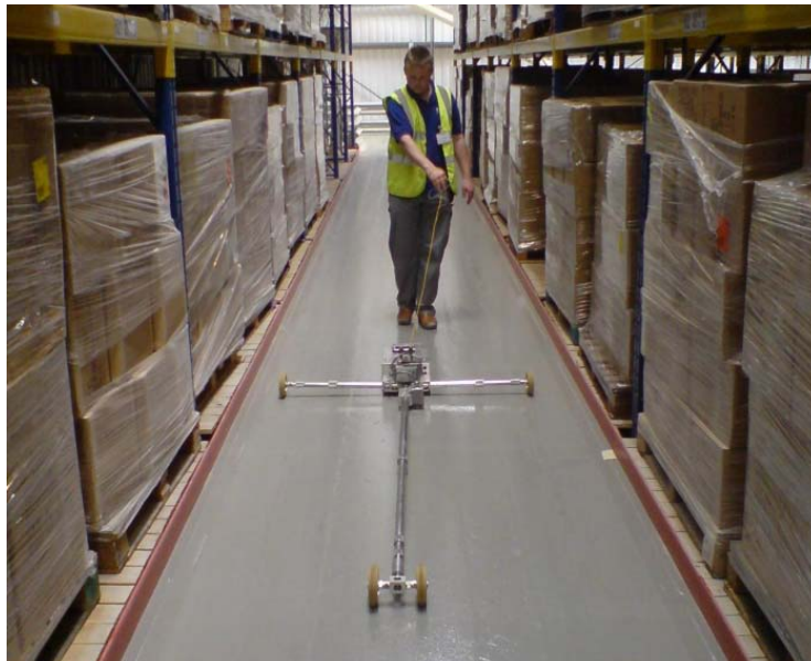
Figure 7: Face Digital Profileograph within a narrow aisle
