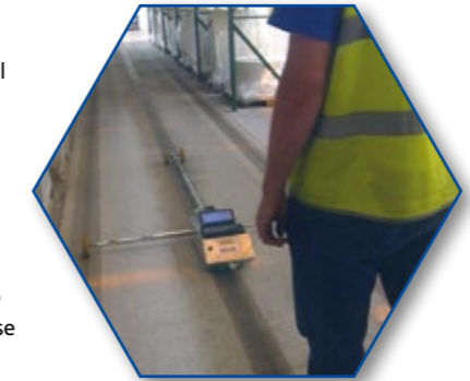
▲ Wheel Base Profilegraph (TR34 / Fmin / EN 15620)
